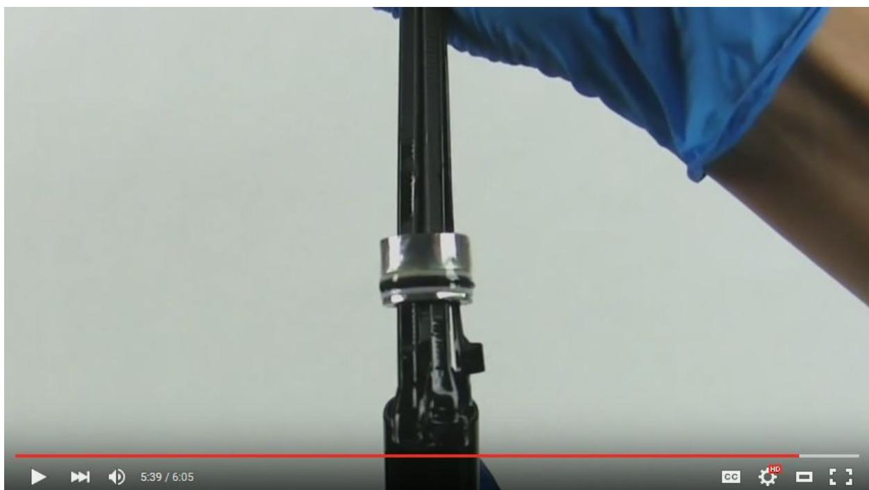
slide the inner seal head from the shaft
