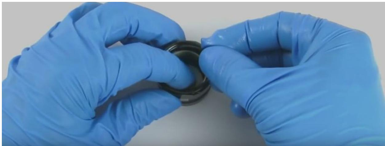
saturate foam ring in reverb oil and install it above the bushing
