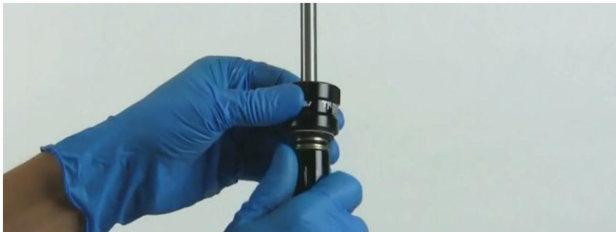
clamp the top tube to the soft jaw vise at the flat section of the post head
