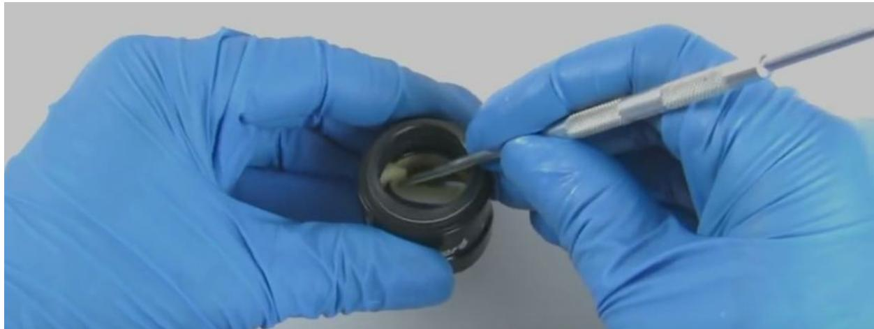
remove the dust wiper with tyre lever
