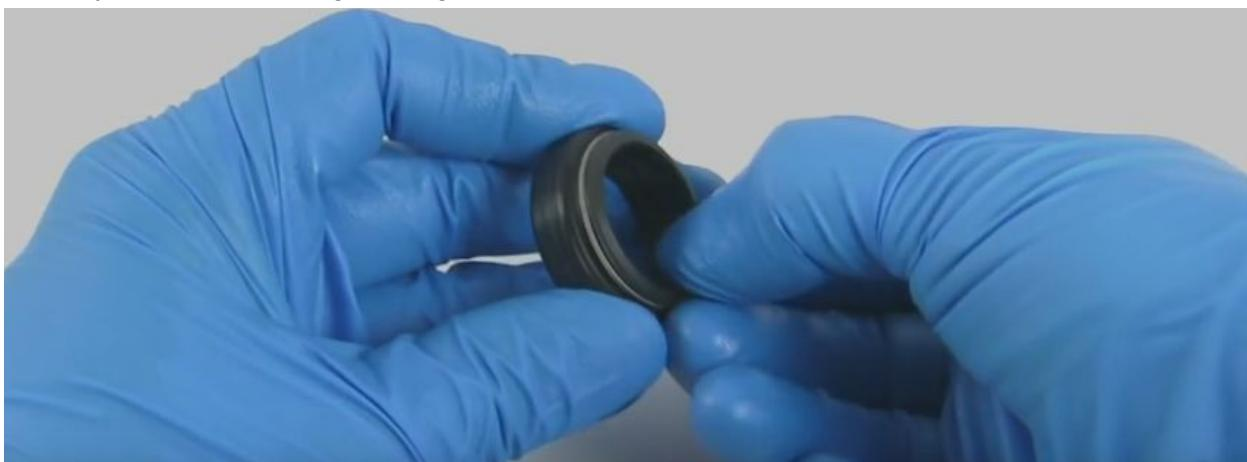
insert the dust wiper into the lower tube
