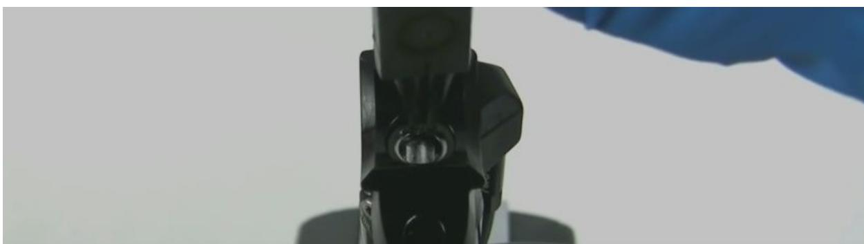
check that the snap ring is properly seated by rotating it back and forth with the snap ring pliers
