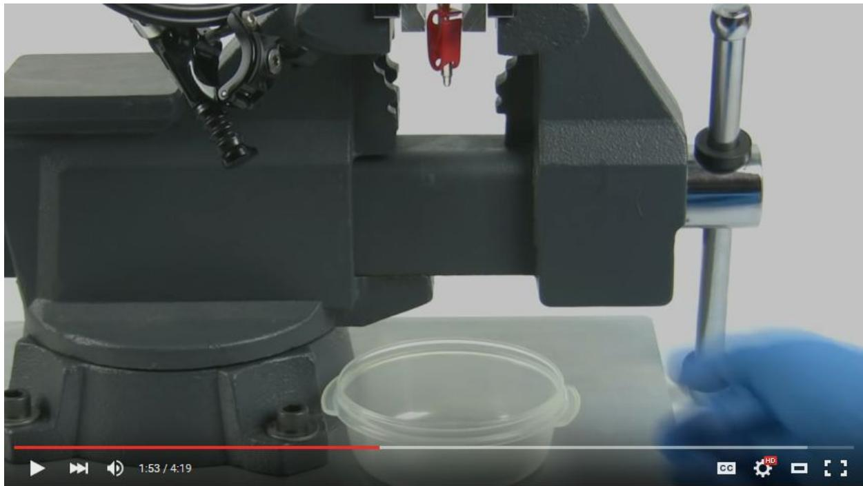
hold the shaft and use the IFP tool to push the IFP to correct depth (100mm for 100mm and 125mm for 125mm posts)
