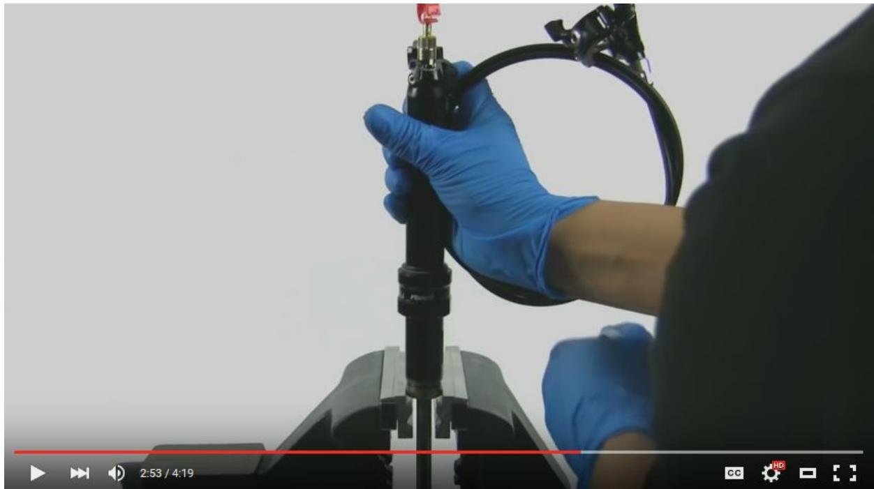
remove the bleed tool and insert oil level tool
