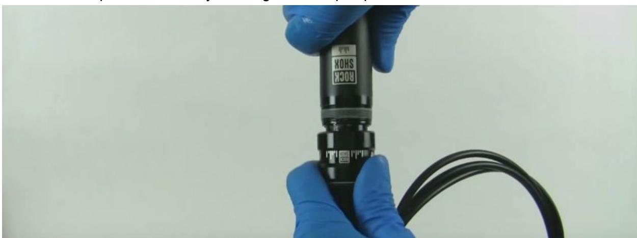
clamp the post to soft jaws below the minimum insertion line, just tight enough to keep the post from spinning
