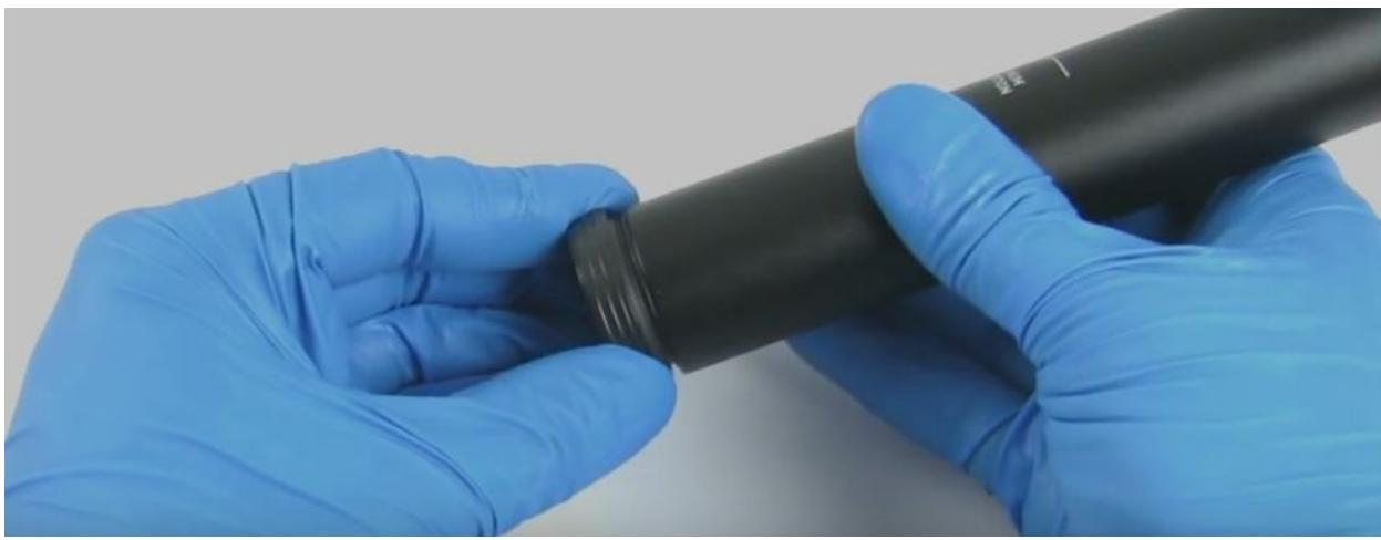
use the lower tube to press the dust wiper into the top cap
