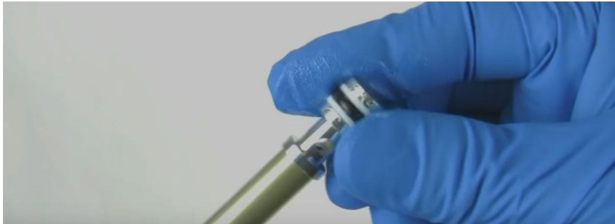
insert shaft piston into the upper post inner tube, just enough for the o-ring to contact the inner tube
