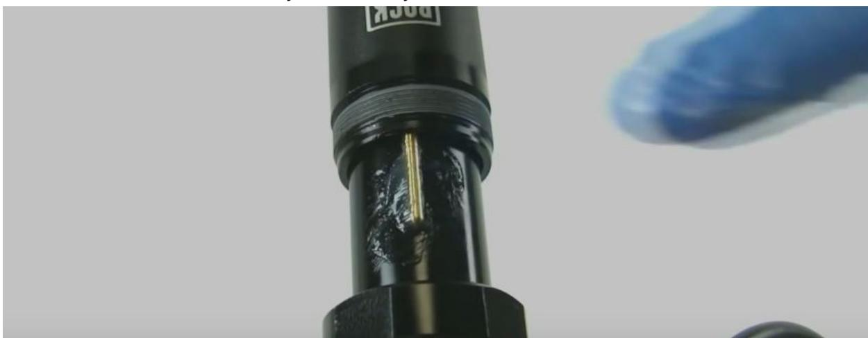
slide the lower post over the keys and against the top cap
