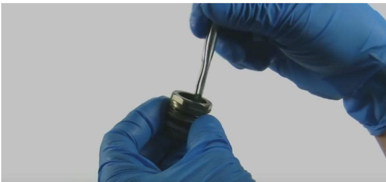
while holding the shaft in place, slide the inner seal head to place and thread it to upper post
