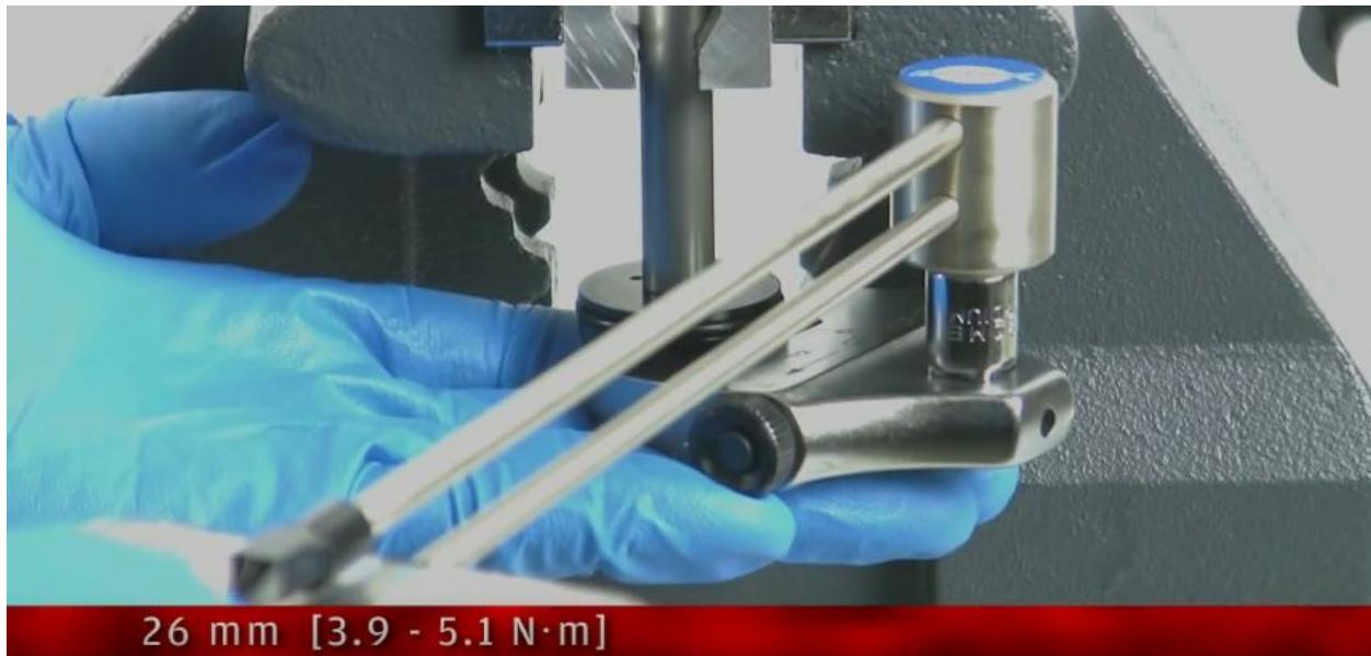
apply small amount of slick honey to schrader valve and install the valve into the outer seal head
