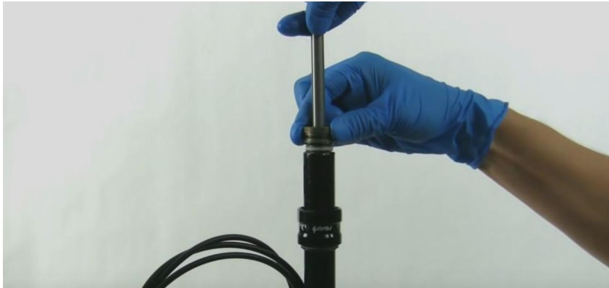
tighten the internal seal head
