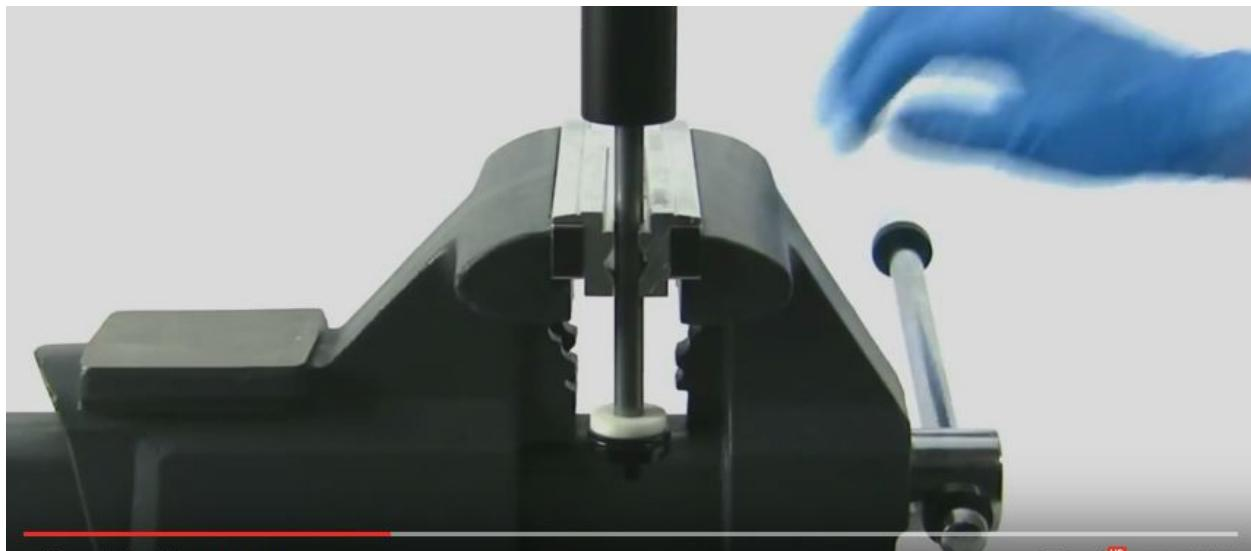
remove outer seal head and foam washer
