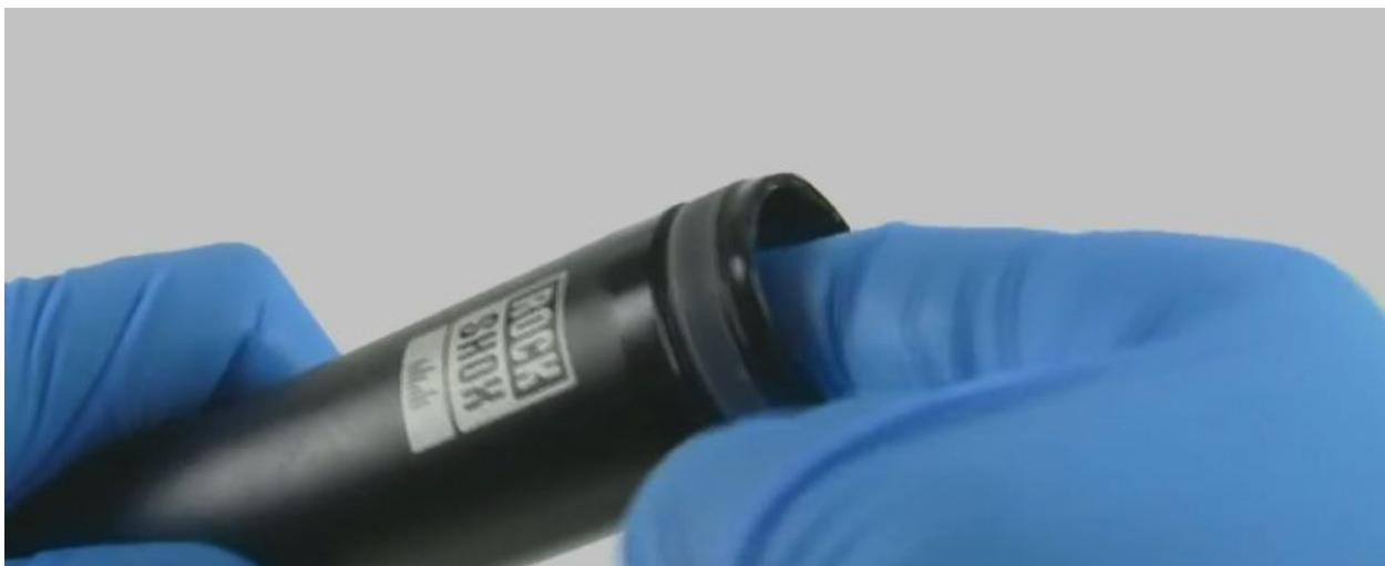
while squeezing the bushing, slide lower post over the upper post until the lowe post starts to cover the key slots
