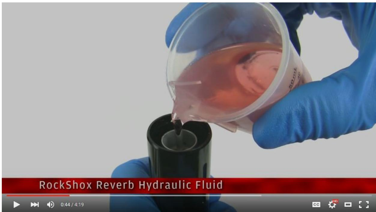
continue to pour until the fluid is level with the top of the post
