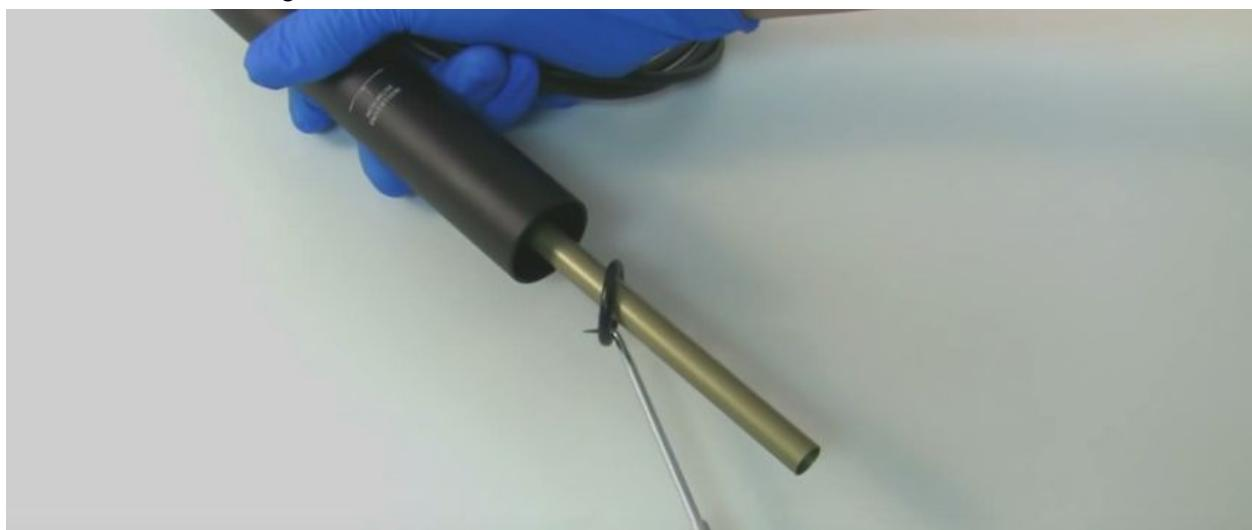
clamp the lower post to soft jaw vice below the minimum insertion line, just enough to keep the post from spinning
