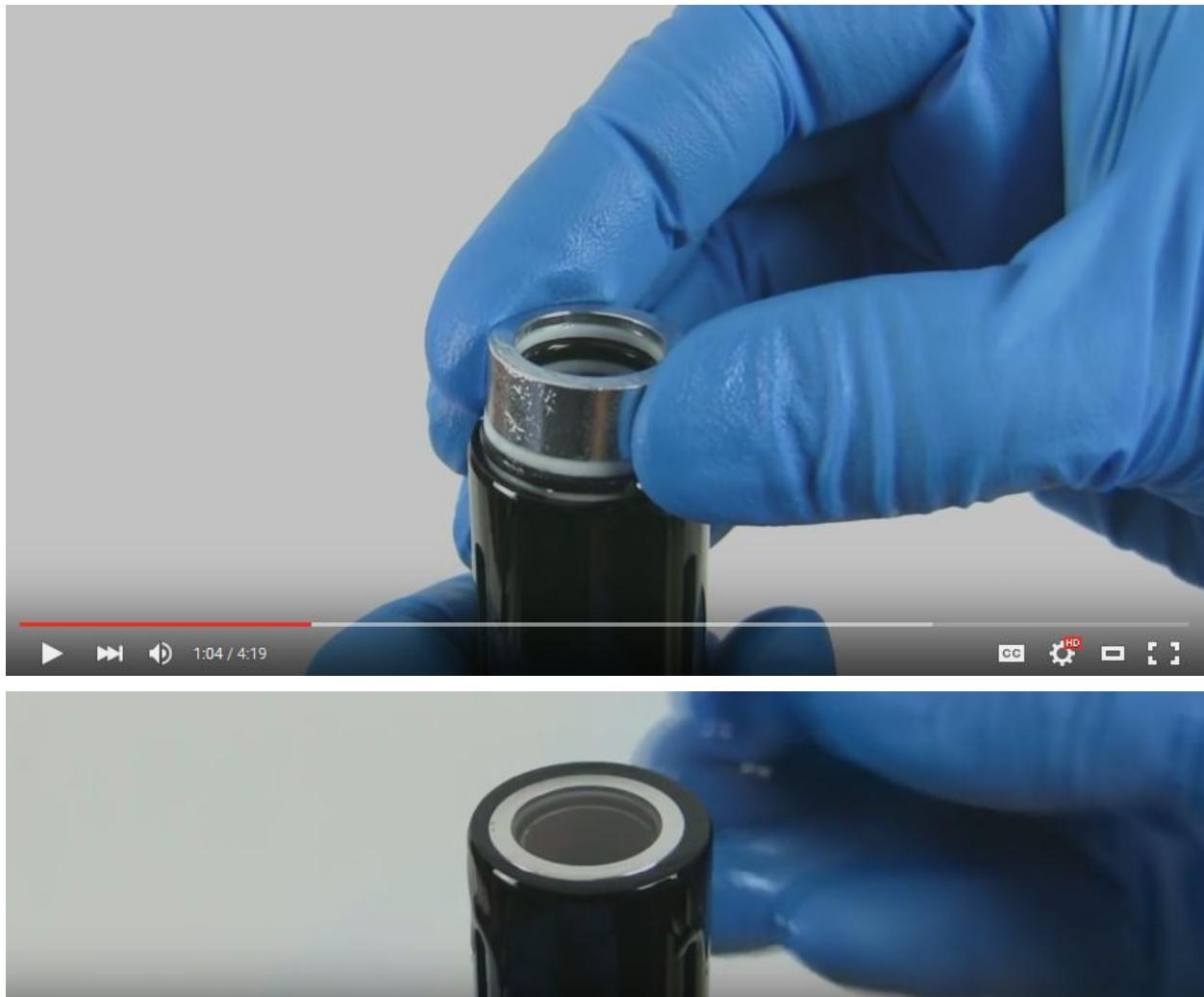
use IFP tool to push the ifp to 10-20mm
