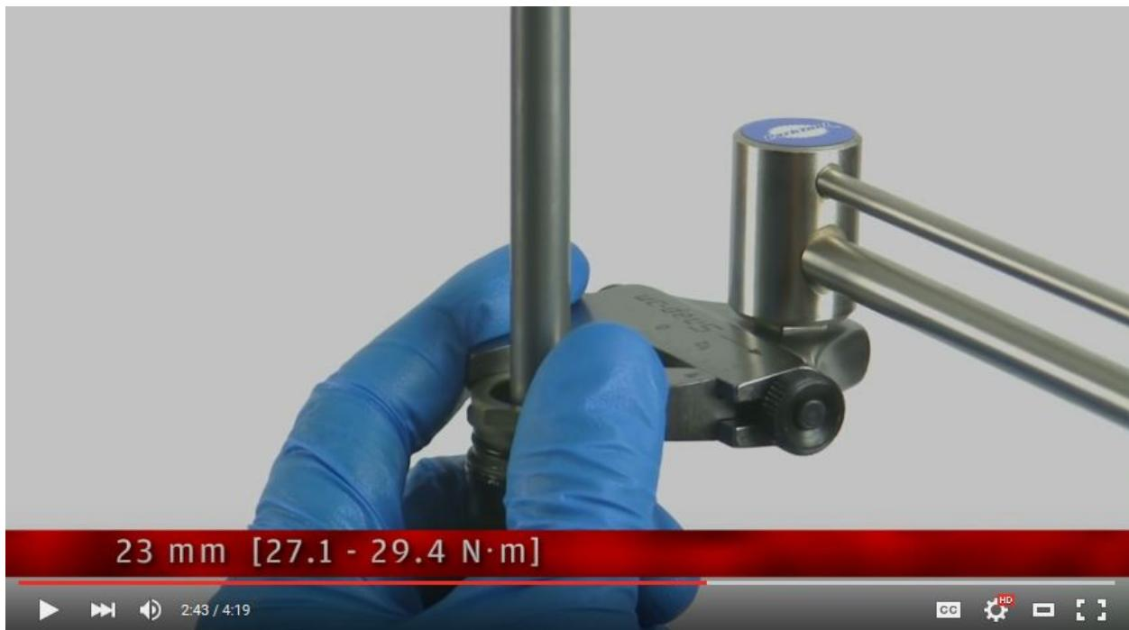
clamp the post from the internal seal head
