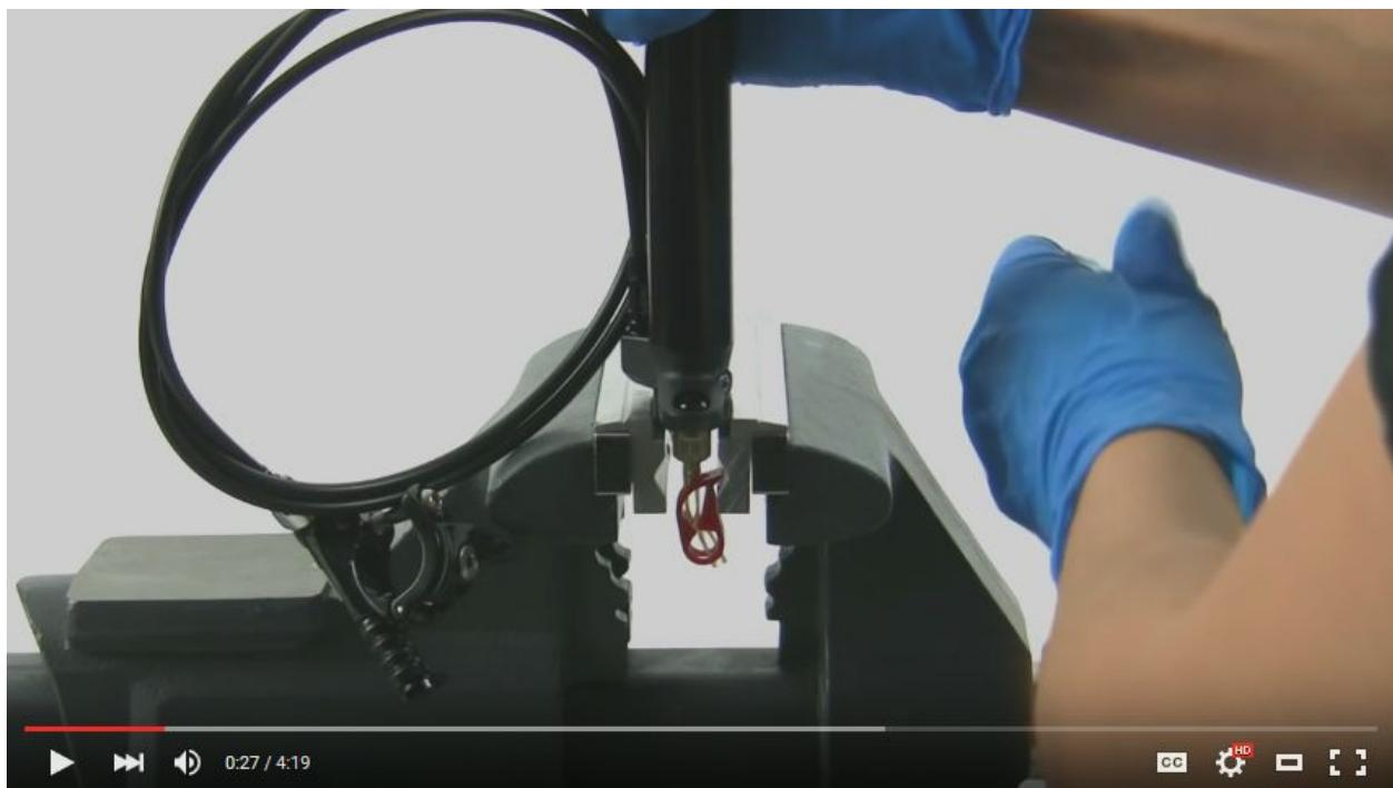
insert the non ported part of the inner tube to the upper post
