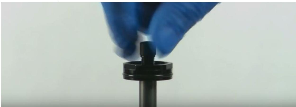
push the lower post over the outer seal head until the snap ring groove is visible
