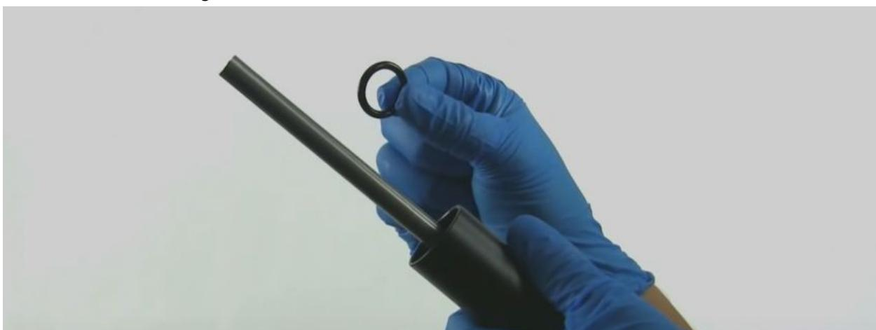
**for 355 and 420mm posts:** apply small amount of slick honey to false bottom insert o-ring and insert the insert into the lower post (orientation, not critical)
