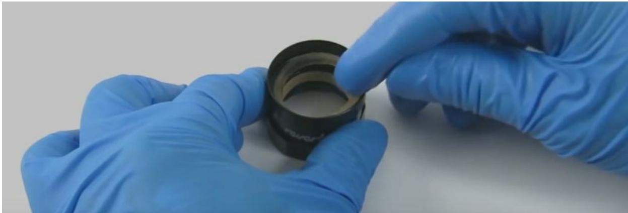
carefully remove the energizer ring from the new dust wiper
