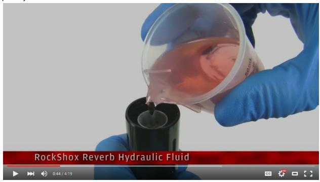
After the inner tube is filled, you can test that the remote works by inserting the piston and pressing it down with and without the remote being pressed. It should not move if remote is not pressed as it enables the oil to flow from inner tube to the post.
