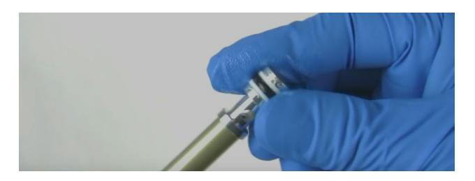
Press the remote and insert shaft piston into the upper post inner tube, so that the piston head stays just above the inner tube. (this will also rise the IFP to it's desired depth)
