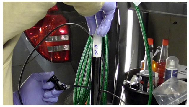
pour additional fluid and again remove the bubbles
