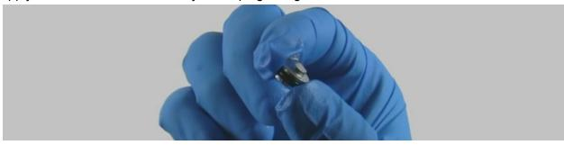
insert the plug into the post head and press firmly until it clears the snap ring groove
