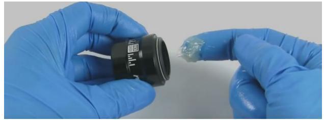
install the top cap to the upper post and slide it until it clears the key slots
