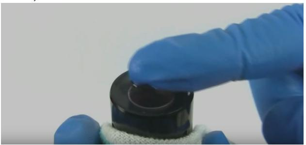
apply small amount of slick honey to internal and external glide- and o-rings of the IFP
