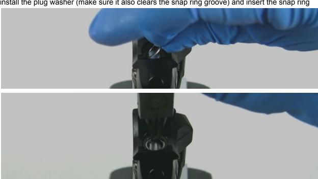
check that the snap ring is properly seated by rotating it back and forth with the snap ring pliers
