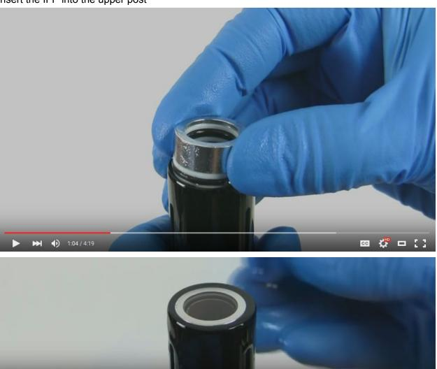
Press the remote to open the pop-it-open-valve and use "IFP tool" to push the ifp to calculated length (132.9mm).
