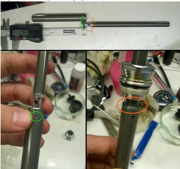
This gave 12mm for piston displacement height, so the volume is  $V = A_{inner\ tube}*h = 111.22mm^2*12mm = 1334.64mm^3$
