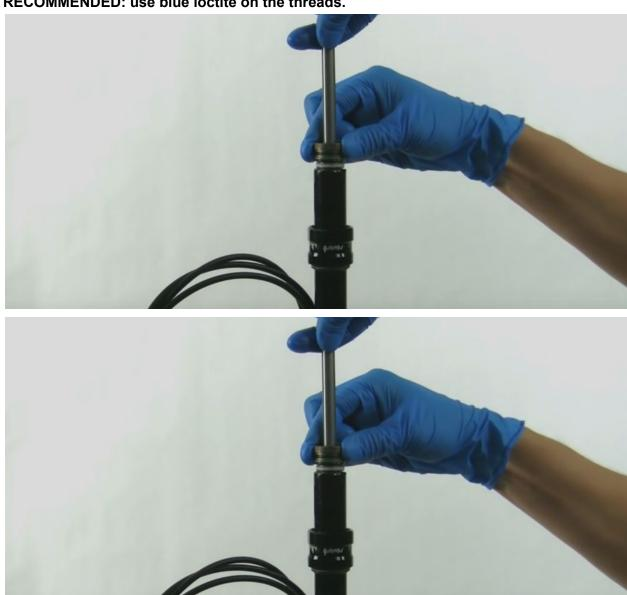
You should feel some resistance before fully threading it (the piston + oil will resist), when this happens, press the remote and fully tighten the inner seal head
