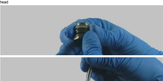
While holding the shaft in place, slide the inner seal head to place and thread it to upper post via hand. (The shaft should be pretty solid as it locked with the oil + pop-open-valve) **RECOMMENDED: use blue loctite on the threads.**
